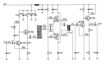
Test circuit for SIP-5 filter Input impedance of the symmetrical post-amplifier: 2 k $\Omega$  in parallel with 3 pF
