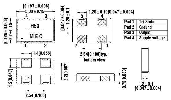
Chamfered pad is pad No. 1. Count counter-clockwise when looking at top view. Count clockwise when looking at bottom view.
