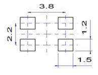
Do not design any conductive path between the pattern
