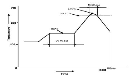
Temperatures are PCB temperatures.
