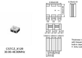
Thickness varies with frequency and built-in capacitance. \*: EIAJ code (in mm)
