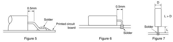
Soldering directly to the case will reduce the degree of vacuum and may result in deterioration of the characteristics and may break the crystal chip.
