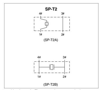
Note: Do not connect terminals #2, #3 of T1A and T2A to the outside electrode. These are dummy terminals.
