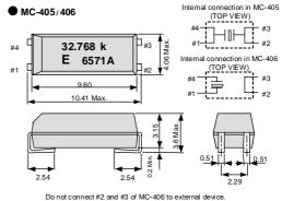
Do not connect #2 and #3 of MC-406 to external device.
