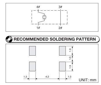
Remarks 1. Do not connect terminals #2, #3 to external device and GND. These are dummy terminals.
