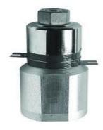
Ultrasonic cleaning transducer can transform high-frequency electrical signals into ultrasonic energy and transfer the energy into the container. The water molecules will be excited to vibrate in a high-frequency and micro-jet also will come into being, thus realizing the non-contact cleaning.
