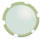
Ultrasonic atomizing transducer is used for ultrasonic atomizer, is one of the main products of Audiowell. This product is made from the piezoelectric ceramic developed by ourselves, has the advantages of better temperature stability and superior piezoelectric effect. It also adopted an advanced membrane technology to protect the electrode, has a good acid and alkali-resistant performance.
