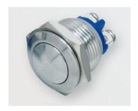
Mounting hole size:Φ16mm Switch rating:3A/250VAC Switch combination:1NO Operation types: Resetable Head shape: Round
