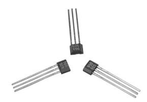
The SS490 Series MRL (Miniature Ratiometric Linear) sensors are small, versatile linear Hall effect devices which are operated by the magnetic field from a permanent magnet or an electromagnet. The ratiometric output voltage is set by the supply voltage and varies in proportion to the strength of the magnetic field.
