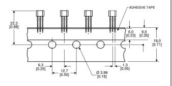
Formed Leads, 14,99 mm [0.59 in]) Long, on Tape SS411A-T2, SS413A-T2, SS441A-T2, SS443A-T2, SS449A-T2, SS461A-T2, SS466A-T2
