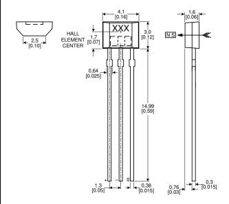
Straight Leads, 18,67 mm [0.735 in] Long SS411A-L, SS413A-L, SS441A-L, SS443A-L, SS449A-L, SS461A-L, SS466A-L
