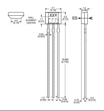
Straight Leads, 14,99 mm [0.59 in]) long, on Tape SS411A-T3, SS413A-T3, SS441A-T3, SS443A-T3, SS449A-T3, SS461A-T3, SS466A-T3
