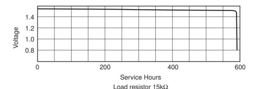
Average Service Capacity: 60 mAh (rated capacity at  $15k\Omega$  load, cut off voltage 1.2V at  $20^{\circ}C$ )
