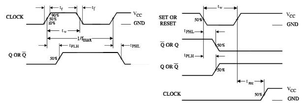
Figure 1. Switching Waveform
