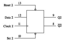
PIN  $14 = V_{CC}$ PIN 7 = GND
