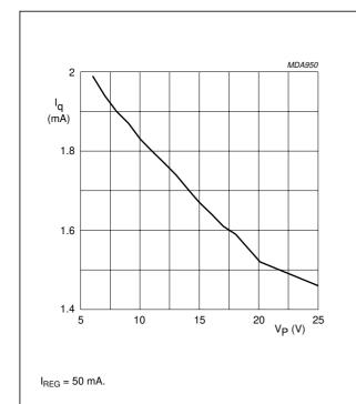
Fig.12 Quiescent current as a function of the supply voltage.
