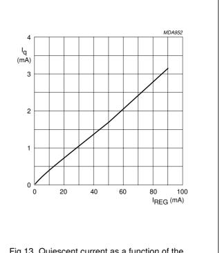
Fig.13 Quiescent current as a function of the output current.
