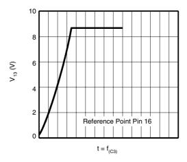
Figure 10-5. Soft-start Voltage (f/V Converter Active)
