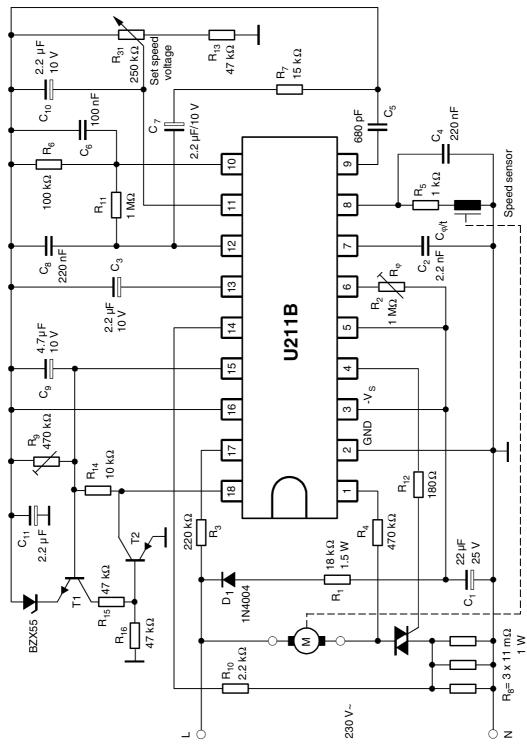
The switch-off level at maximum load shows in principle the same speed dependency as the original version (see Figure 10-17 on page 21), but when reaching the maximum load, the motor is switched off completely. This function is effected by the thyristor (formed by  $T_1$  and  $T_2$ ) which ignites when the voltage at pin 15 reaches typically 7.4 V (reference point pin 16). The circuit is thereby switched to standby mode over the release Pin 18.
