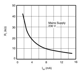
Figure 10-15. Power Dissipation of R<sub>1</sub>
