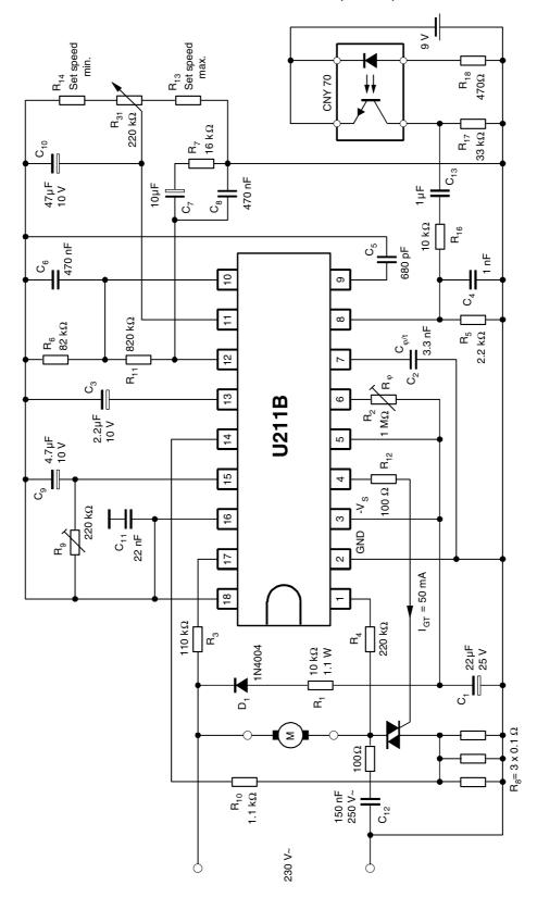
The schematic diagram (see Figure 10-22 on page 26) is designed as a speed control IC based on the reflection-coupled principle with 4 periods per revolution and a maximum speed of 30000 rpm. The separation of the coupler from the rotating aperture should be about approximately 1 mm. In the schematic diagram, the power supply for the coupler was provided externally because of the relatively high current consumption.
