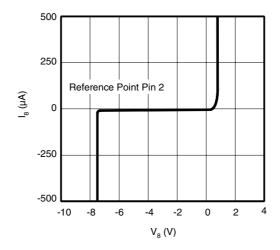
Figure 10-8. Amplifier Output Characteristics
