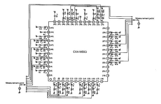
Fig 6. Audio system (output DC offset)
