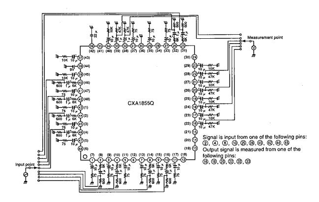
Fig 3. Audio system (gain, frequency response characteristics, total harmonic distortion, input dynamic range)
