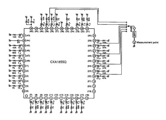
Fig 7. Audio system (residual noise)
