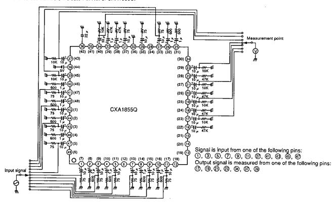
Fig 1. Video system (gain, frequency response characteristics, input dynamic range)
