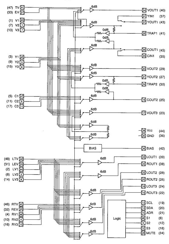
Note) A total gain of 0dB is achieved by connecting a  $6k\Omega$  resistor to the each audio input.
