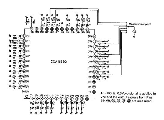
Fig 5. Audio system (ripple rejection)
