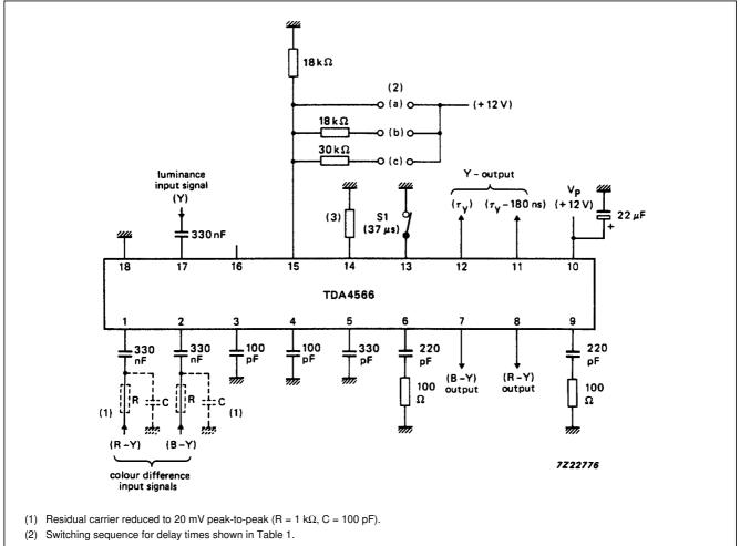
(3) R<sub>14–18</sub> = 1.2 k $\Omega$  for TDA4566. R<sub>14–18</sub> = 1.15 k $\Omega$  for TDA4566A (27 k $\Omega$  resistor connected in parallel to 1.2 k $\Omega$ ).
