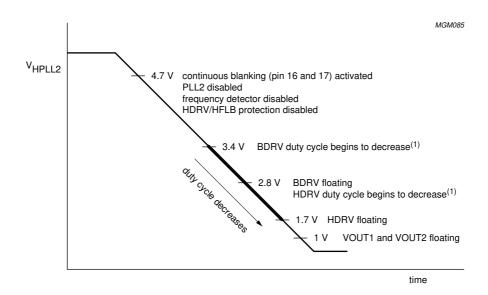
b. PLL2 soft-down sequence, via the  $I^2C$ -bus, if  $V_{CC} > 8.6 \text{ V}$ .
