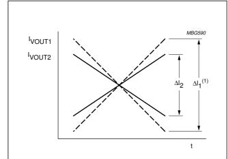
∆I<sub>1</sub> is the maximum amplitude setting at register VSIZE = 127, control bit VOVSCN = 0, control bit VPC = 1, control bit VSC = 1 and control bit VLC = 1.
