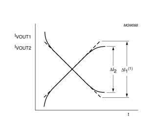
(1)  $\Delta I_1$  is the maximum amplitude setting at register VSIZE = 127, register VOVSCN = 0, control bit VPC = 1, control bit VLIN = 1 and control bit VLINBAL = 0.
