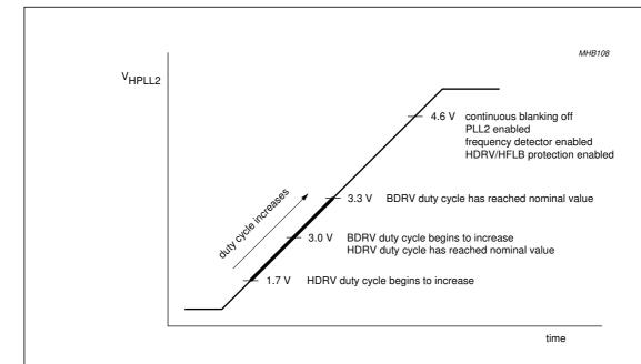
a. PLL2 soft start sequence by external DC current, if  $V_{CC} > 8.6 \text{ V}$ .
