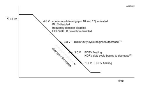
b. PLL2 soft-down sequence by external DC current, if  $V_{CC} > 8.6 \text{ V}$ .
