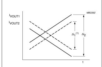
(1)  $\Delta I_1$  is the maximum amplitude setting at register VSIZE = 127 and control bit VPC = 1.
