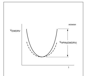
Fig.9 Adjustment of parabola amplitude at pin EWDRV.
