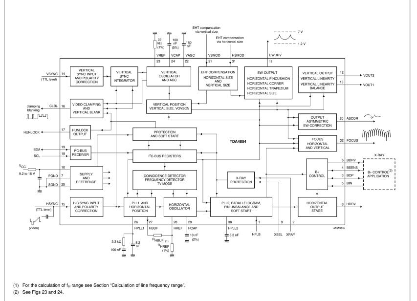
Fig.2 Block diagram and application circuit of TDA4854.
