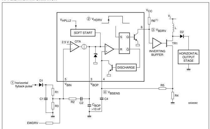
For f < 50 kHz and C2 < 47 nF calculation formulas and behaviour of the OTA are the same as for an OP. An exception is the limited output current at BOP (pin 3). See Chapter "Characteristics", Row Head "B+ control section; see Figs 23 and 24".
