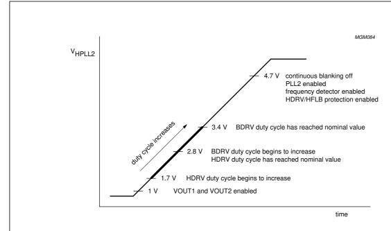
a. PLL2 soft start sequence, via the  $I^2C$ -bus, if  $V_{CC} > 8.6 \text{ V}$ .
