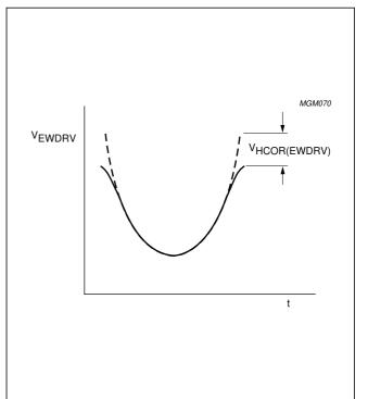
Fig.10 Influence of corner correction at pin EWDRV.
