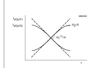
(1)  $\Delta I_1$  is the maximum amplitude setting at register VSIZE = 127 and VLIN = 0%.
