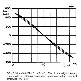
Fig.12 Control range of S correction.
