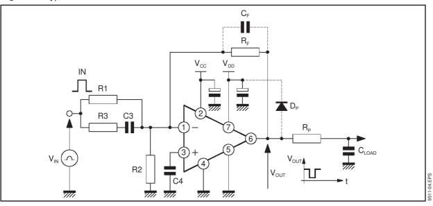
$\begin{array}{l} \mbox{Recommended values}: \\ \mbox{R1} = 1 k \Omega, \mbox{R2} = 1.8 k \Omega, \mbox{R}_{F} = 20 k \Omega, \mbox{R}_{P} = 200 \Omega, \\ \mbox{C4} > 10 n F, \mbox{ C3} = 10 \mbox{ to } 12 p F \mbox{ for } C_{F} \mbox{ \# } 0.5 p F. \\ \mbox{R3} \mbox{ \# } 150 \Omega. \end{array}$
