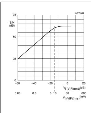
Fig.5 Typical signal-to-noise ratio as a function of IF input voltage.
