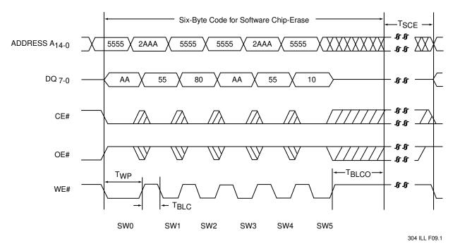
FIGURE 10: SOFTWARE CHIP-ERASE TIMING DIAGRAM
