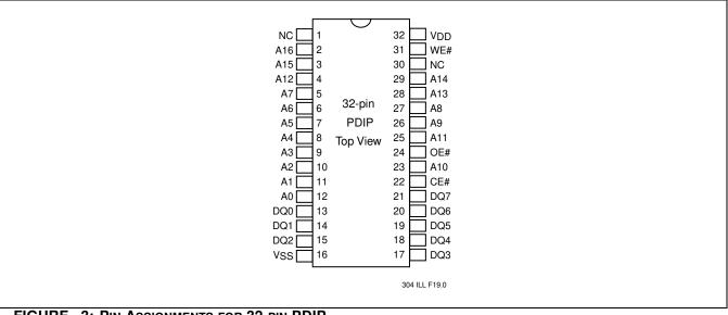
FIGURE 3: PIN ASSIGNMENTS FOR 32-PIN PDIP
