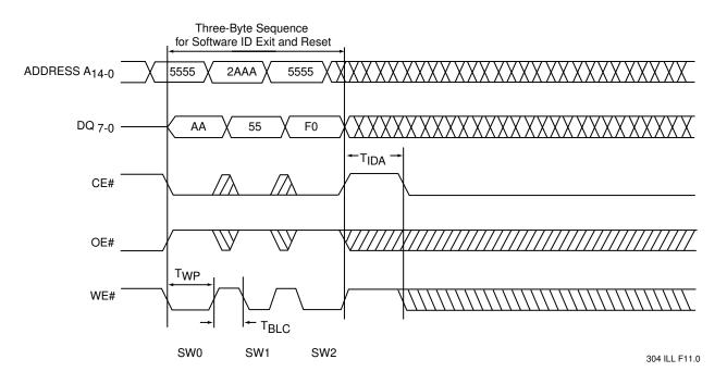
FIGURE 12: SOFTWARE ID EXIT AND RESET
