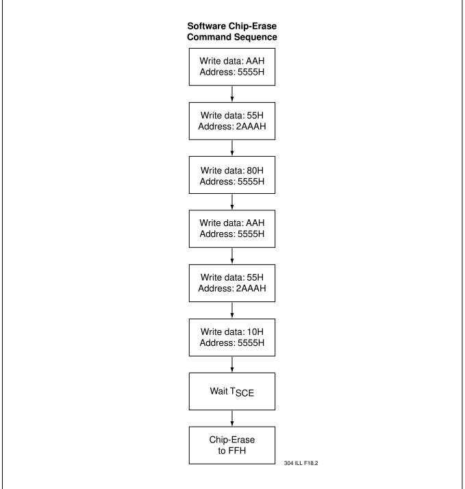
FIGURE 19: SOFTWARE CHIP-ERASE COMMAND CODES
