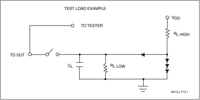
FIGURE 14: A TEST LOAD EXAMPLE
