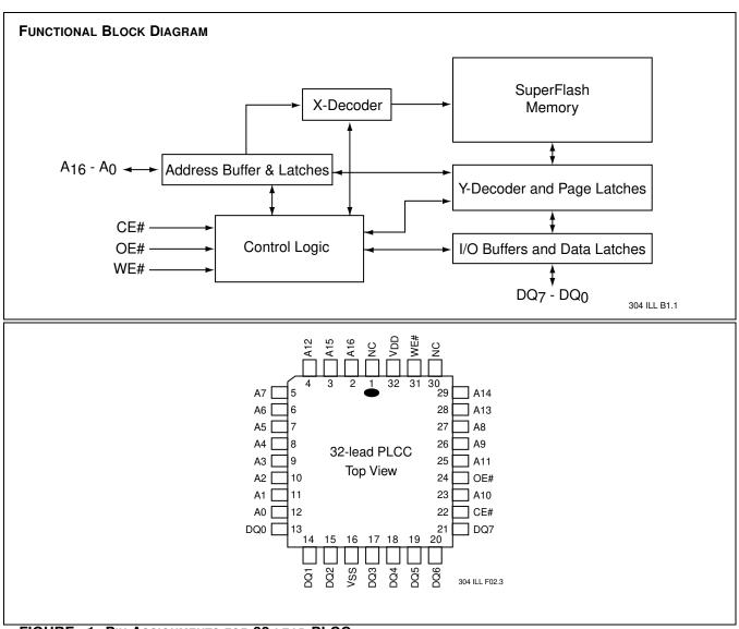
FIGURE 1: PIN ASSIGNMENTS FOR 32-LEAD PLCC
