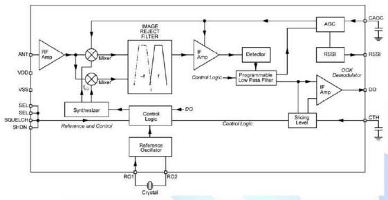
Figure 1, CY520 Simplified Block Diagram
