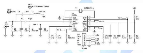
Figure 3. CY520 Application Example, 433.92 MHz
