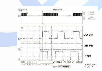
Figure 11. Time to Good Data, External Oscillator, Room Temperature.
