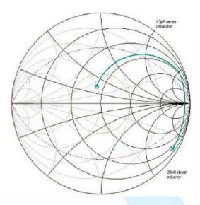
Figure 5. Plotting the Shunt Inductor and Series Capacitor
