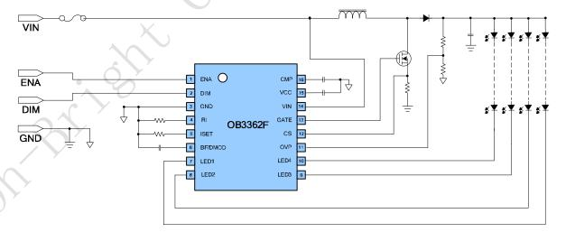
Figure 1: OB3362F Typical Application Schematic
