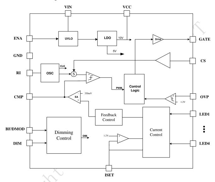
Figure2: OB3362F Functional Block Diagram
