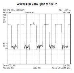
433.92MHz Phase Noise, ASK = CW, 1MHz Offset, -78.49dBc/Hz
