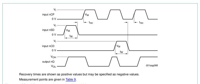
Fig 5. nSD, nCD recovery time and pulse width
