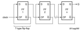
Fig 8. Binary ripple up-counter; divide-by-2<sup>n</sup>
