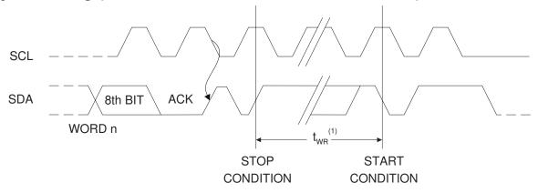
Note: 1. The write cycle time t<sub>WR</sub> is the time from a valid stop condition of a write sequence to the end of the internal clear/write cycle.
