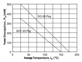
Figrue 9. Power Derating Curve
