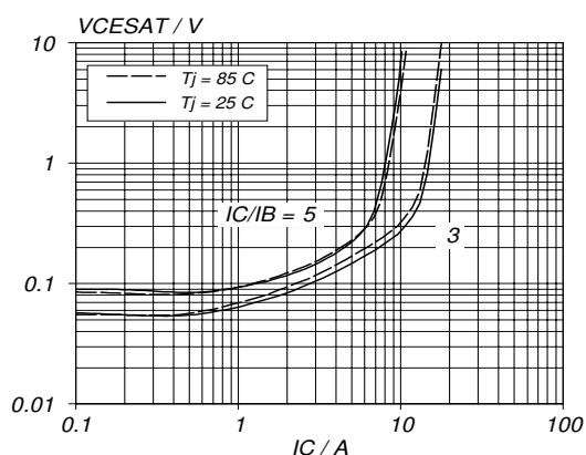
Fig.9. Typical collector-emitter saturation voltage.
