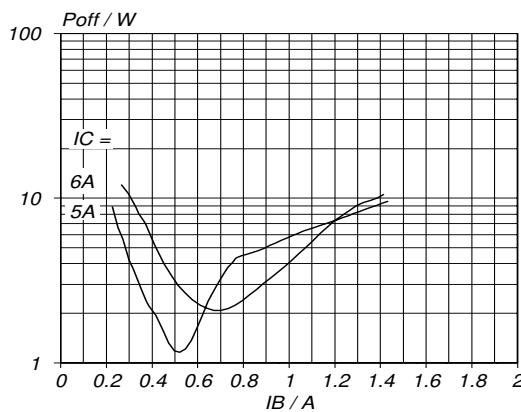
Fig.11. Typical turn-off losses.  $T_j = 85\text{ }^\circ\text{C}$
