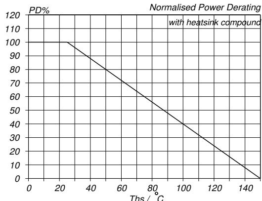
Fig.13. Normalised power dissipation.
