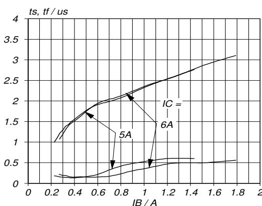
Fig.12. Typical collector storage and fall time.
