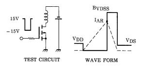
$$\begin{array}{ll} R_G \!=\! 25\Omega \\ V_{DD} \!=\! -50 V, \; L \!=\! 6.3 mH \end{array} \qquad E_{AS} \!=\! \frac{1}{2} \cdot L \cdot I^2 \cdot (\frac{B_{VDSS}}{B_{VDSS} - V_{DD}}) \end{array}$$
