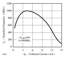
Figure 2. Transition Frequency vs. Collector Current
