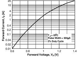
Figure 2. Forward Voltage Characteristics
