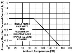
Figure 1. Forward Current Derating Curve
