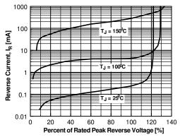
Figure 4. Reverse Current vs Reverse Voltage
