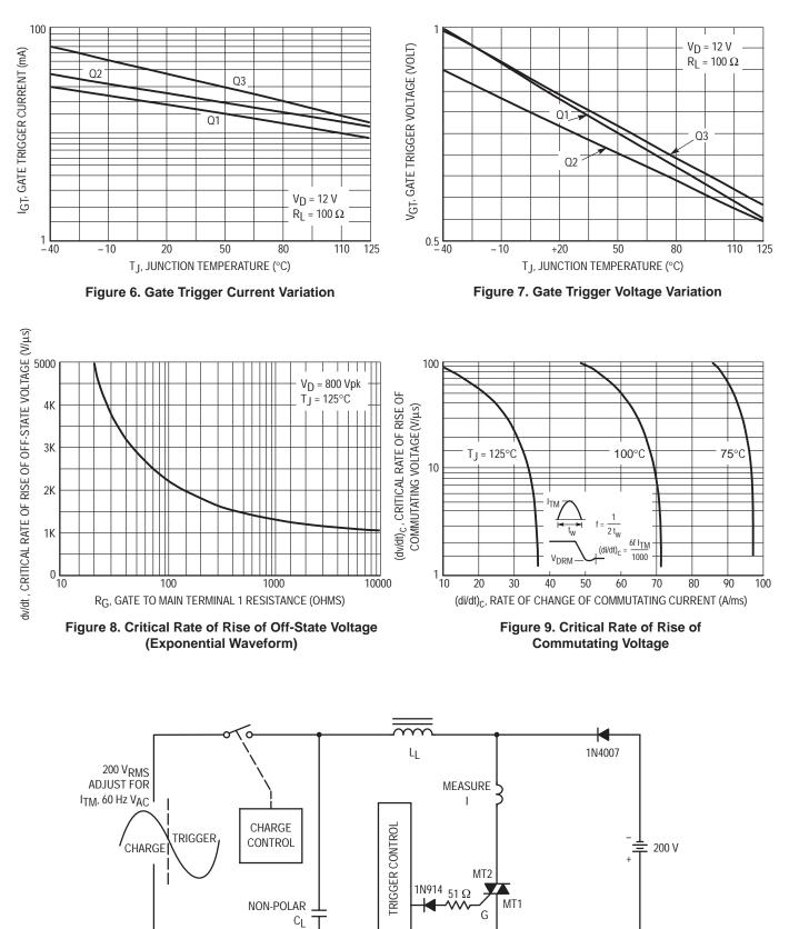
Note: Component values are for verification of rated (di/dt)<sub>C</sub>. See AN1048 for additional information.
