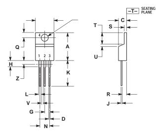
NOTES: 1. DIMENSIONING AND TOLERANCING PER ANSI Y14.5M, 1982. 2. CONTROLLING DIMENSION: INCH. 3. DIMENSION Z DEFINES A ZONE WHERE ALL BODY AND LEAD IRREGULARITIES ARE ALLOWED.
