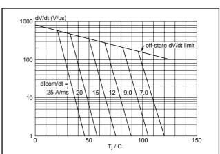
Fig.12. Typical commutation dV/dt versus junction temperature, parameter commutation dl<sub>1</sub>/dt. The triac should commutate when the dV/dt is below the value on the appropriate curve for pre-commutation dl<sub>1</sub>/dt.
