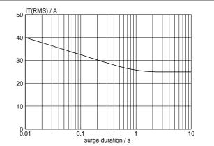
Fig.5. Maximum permissible repetitive rms on-state current  $I_{T(RMS)}$ , versus surge duration, for sinusoidal currents, f = 50 Hz;  $T_{mb} \le 91$  °C.
