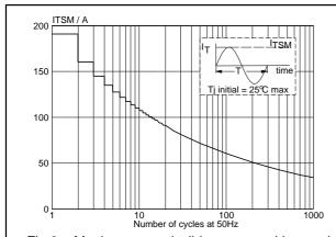
Fig.3. Maximum permissible non-repetitive peak on-state current  $I_{\text{TSM}}$ , versus number of cycles, for sinusoidal currents, f = 50 Hz.
