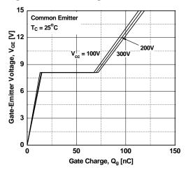
Figure 12. Turn-on Characteristics vs.
