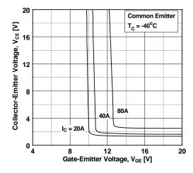
Figure 7. Saturation Voltage vs. V<sub>GE</sub>
