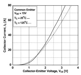
Figure 5. Saturation Voltage vs. Case
