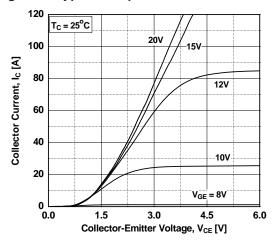
Figure 3. Typical Saturation Voltage Characteristics
