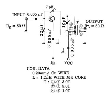
Figure 1 45 MHz Gpe Test Circuit
