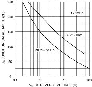
Fig. 5 Typical Junction Capacitance
