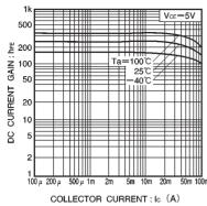
Fig.1 DC current gain vs. collector current
