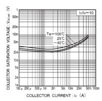
Fig.2 Collector-emitter saturation voltage vs. collector current
