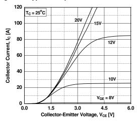
Figure 3. Typical Saturation Voltage Characteristics
