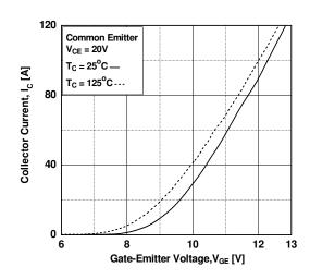
Figure 6. Saturation Voltage vs. V<sub>GE</sub>
