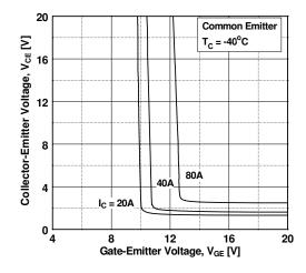
Figure 7. Saturation Voltage vs. V<sub>GE</sub>
