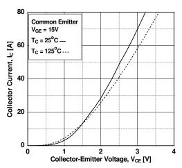
Figure 5. Saturation Voltage vs. Case
