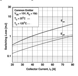
Figure 14. Turn-on Characteristics vs.
