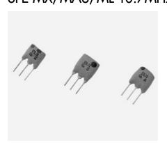
The SFE 10.7MX/MA8/ML lines of ceramic filters were designed to minimize the dispersion of amplitude and phase characteristics within the pass band. Because the excellent G.D.T. characteristics of these filters insure signal integrity, they are recommended for use in applications ranging from high grade stereo receivers to digital transmission systems.
