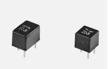
The CFUS Y lines of ceramic filters are 4-element devices connected in ladder form while the CFWS Y455 filters contain 6-elements. These highly selective filters are designed to address the G.D.T. characteristics required in digital communications. The excellent G.D.T. characteristics allow these filters to be utilized in areas such as the mobile cellular markets as well as a variety of stereo applications. Available in 450kHz and 455kHz versions.
