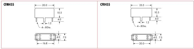
Note: For safety purposes, connect the output of filters to the IF amplifier through a DC blocking capacitor. Avoid applying a direct current to the output of ceramic filters.
