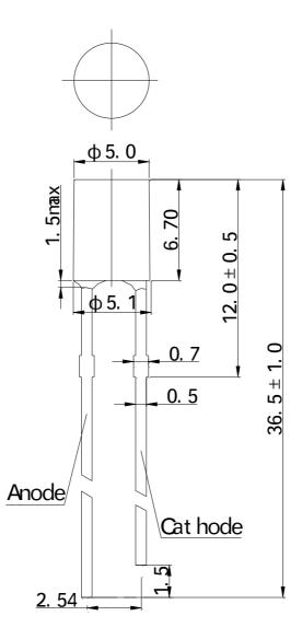
All dimensions in mm, tolerances unless mentioned is  $\pm 0.2$  mm.
