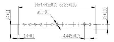
Fig.4 Punching pattern seen from solder side
