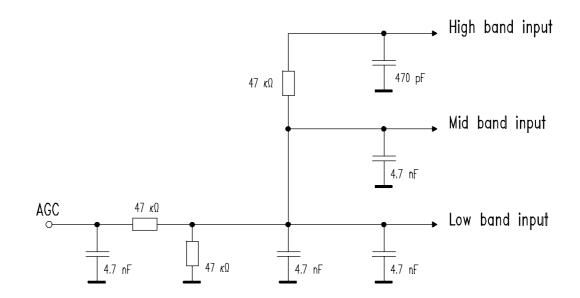
Fig.2 Internal AGC circuit.
