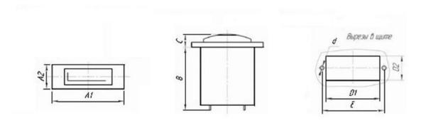
A1 - 54mm, A2 - 21mm, B - 44mm, C - 12mm, D1 - 40,5mm, D2 - 21mm, d - 3,4mm, E - 46mm.
