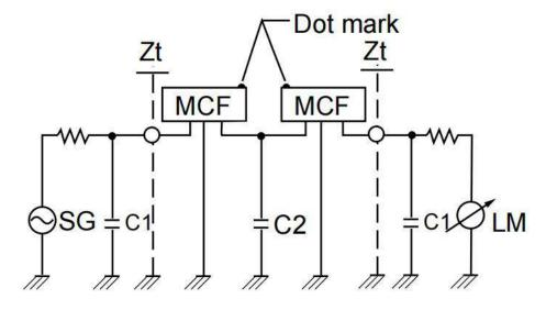
4-POLE MCF Zt: Terminating Impedance
