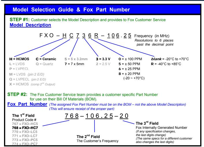
This example, FXO-HC736R-106.25 = HCMOS Output, Ceramic 7 x 5mm Package, 3.3V,  $\pm 25$  PPM Stability, -40 to +85°C Temperature Range, at 106.25 MHz
