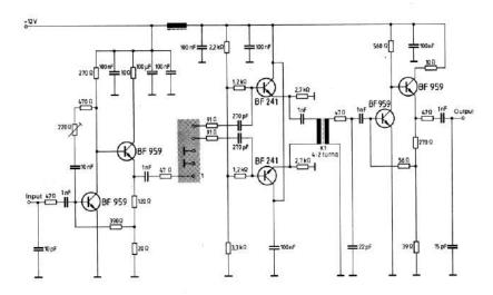
Test circuit for SIP-5 filter Input impedance of the symmetrical post-amplifier: 2 k $\Omega$  in parallel with 3 pF
