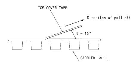
[Figure 1] Carrier Tape Dimensions
