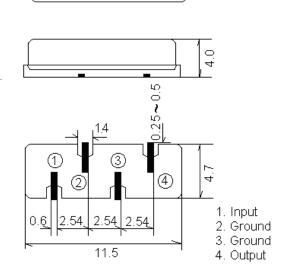
■Recommended layout of PCB(MM) (Tolerance ± 0.2MM)
